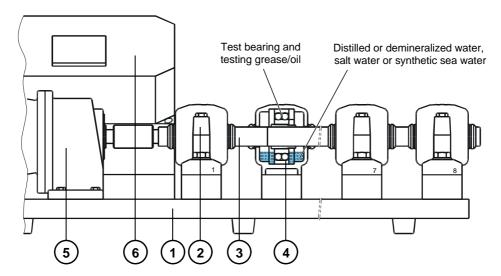
The SKF TMG/EMCOR Grease Testing Machine consists of a ground plate 1 on which eight polyamid housings 2 are mounted. A with a nylon coating protected shaft 3 carries the test bearings 4 and is driven by an electric motor 5. An electronic clock 6 controls the running/stopping periods.
