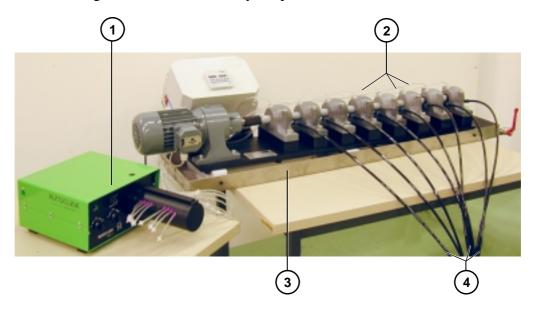
The SKF TMG/EMCOR for the washout test is the same device as the standard EMCOR (as described before) with some options like the peristaltic pump 1 feeding and outlet pipes 2 and 4 and overflowing container 3. The mechanics is inclined so that an angle from the horizontal of 1.5° is formed and
